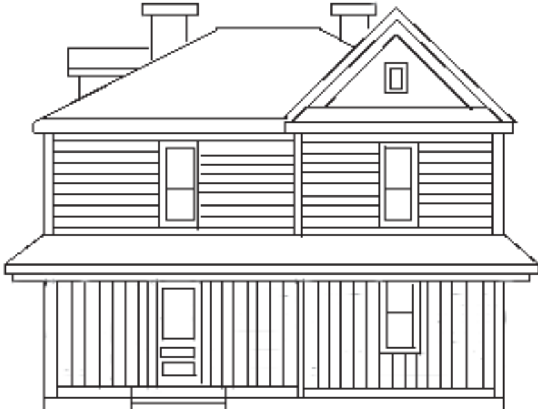
Inappropriate Siding should be applied horizontally.
