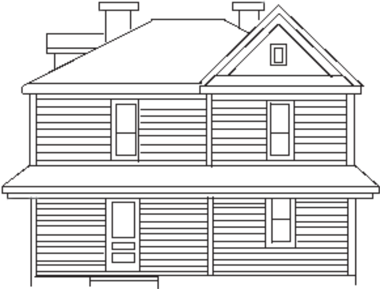
Appropriate Siding should be replaced with materials which duplicate the original in size, shape, and texture.
